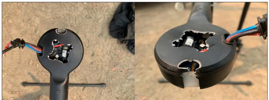
**Figure 2: Motor mount after departure of motor.**
