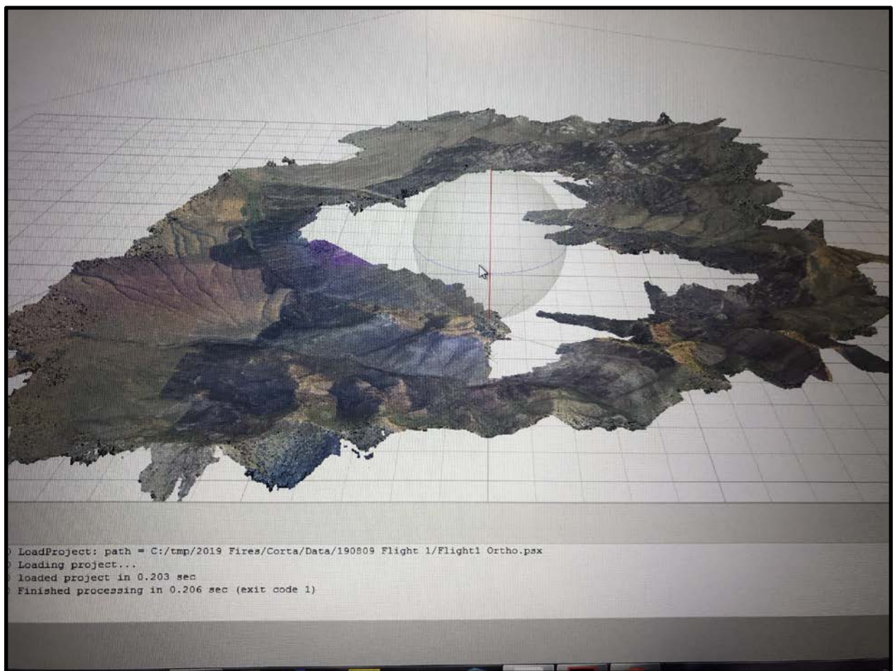
Example of a dense point cloud used to derive imagery for fire perimeter/fire effects
