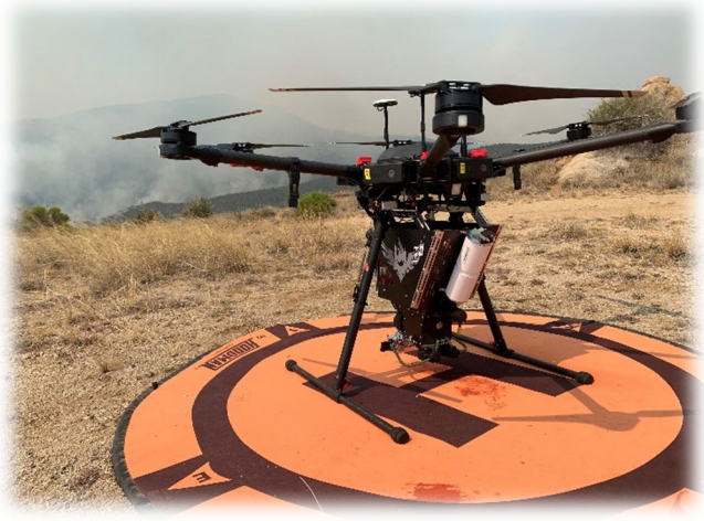
DJI M600 with IGNIS 2.0 Aerial Ignition Payload
